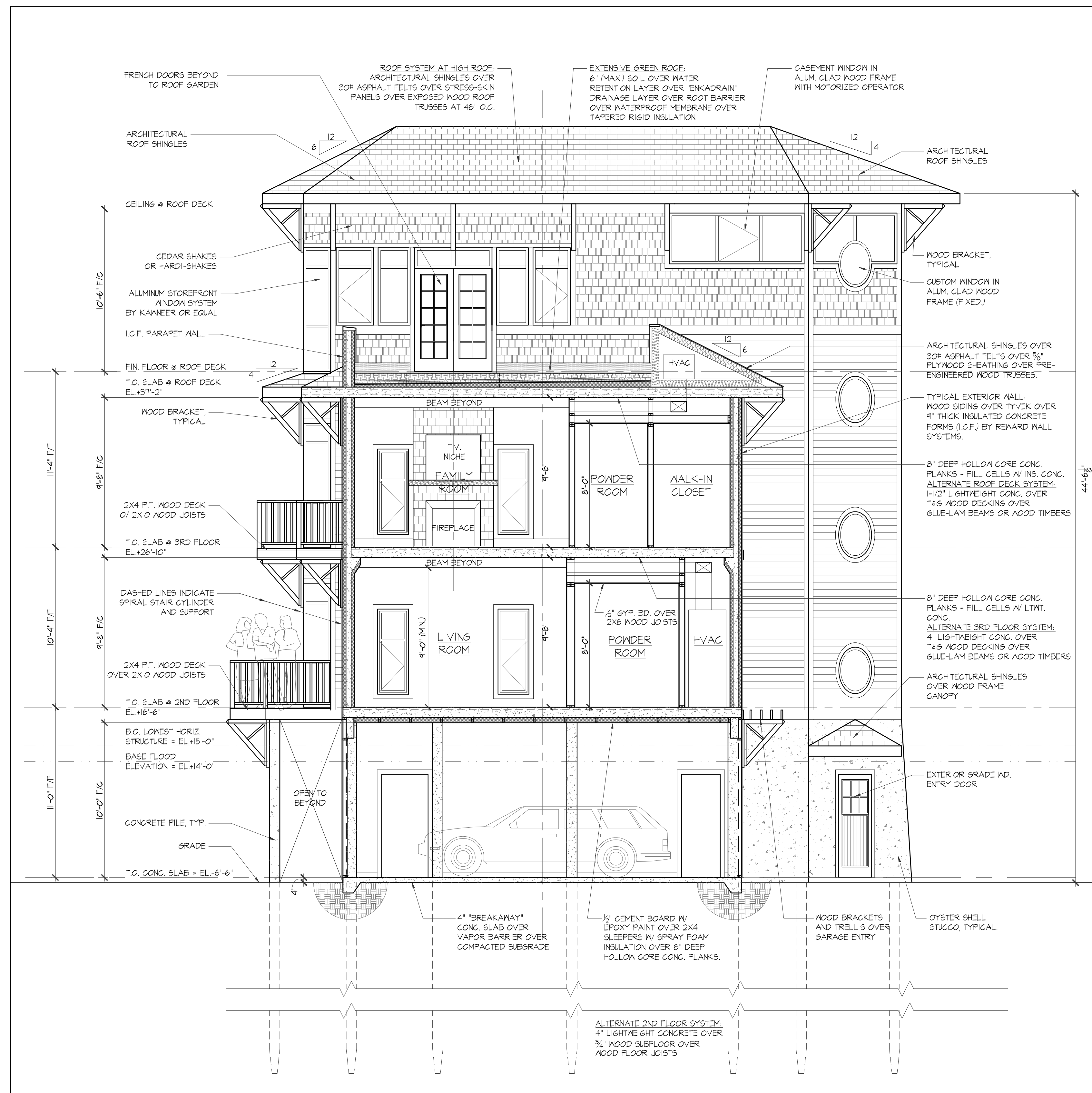
1 TRANSVERSE BUILDING SECTION 1/4" = 1'-0"
